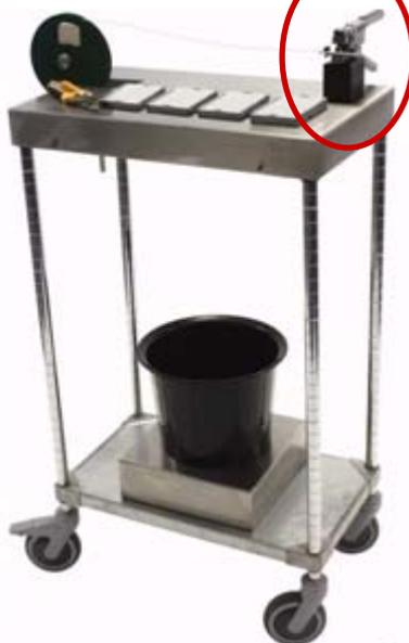
mounted on wheels for portability, which have brakes for increased safety. The trolley and all its various pieces are completely ESD safe.
